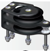
MOD. 00812 DOUBLE FOOT WEIGHT** – 0.57 kg • SWL – 2200 kg SCREWS – 4xØ8 mm (included)
